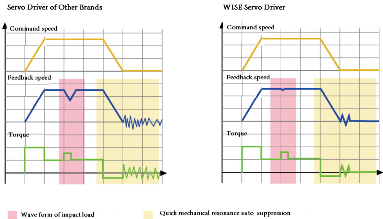
Fig. 1-5 Comparison between counterparts and WISE servo driver
