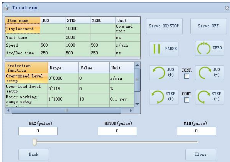
Fig. 3-27 Trial run window-running
