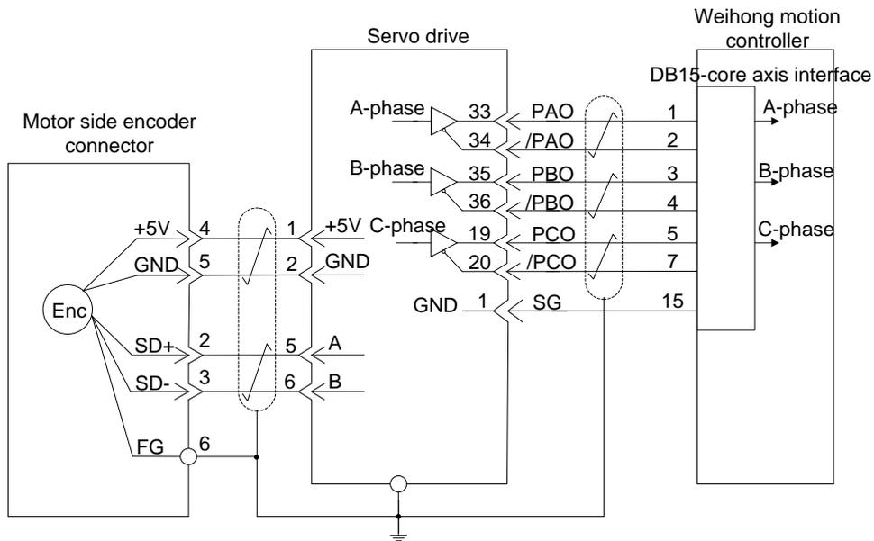
Below is the wiring diagram of MDME model motor (1000W and 1500W) with 20-bit incremental encoder.
