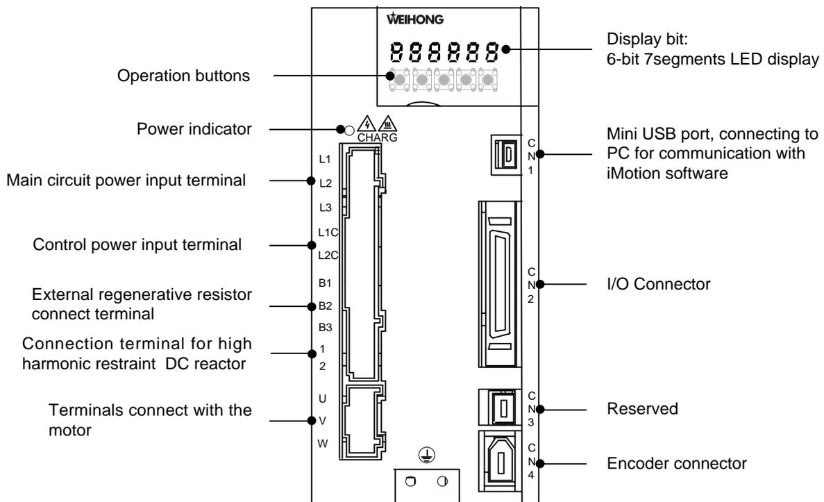
Fig. 1-1 Part description of a non-bus driver
