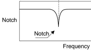
Adjust the frequency, width and depth of the notch filter:
