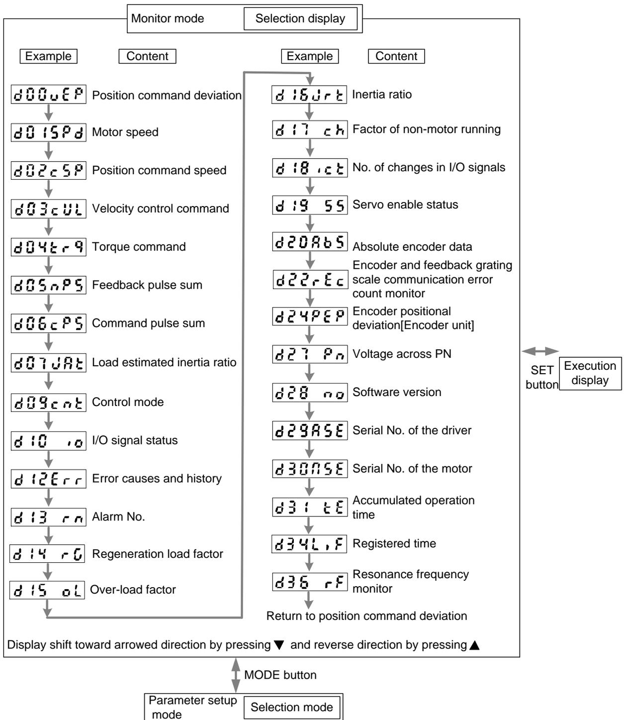
You can press SET button after monitor mode is selected by pressing MODE button, to access following options. When a certain option is accessed, press SET button to view and execute the concrete content; press SET button again to return to “Selection display”.
