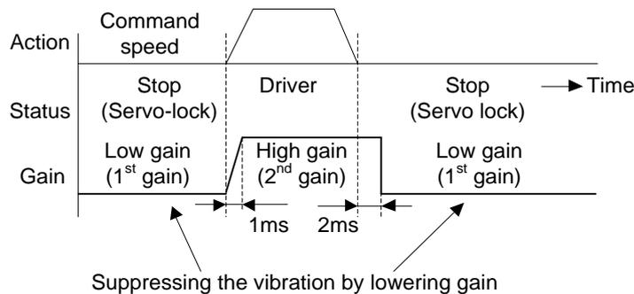
In example below, you can reduce the noise at motor at stalling (servo lock) by setting up to lower gain after the motor stops. Please refer to section 6.2.4 “Basic Gain Parameter Setup Table” to make adjustment.
