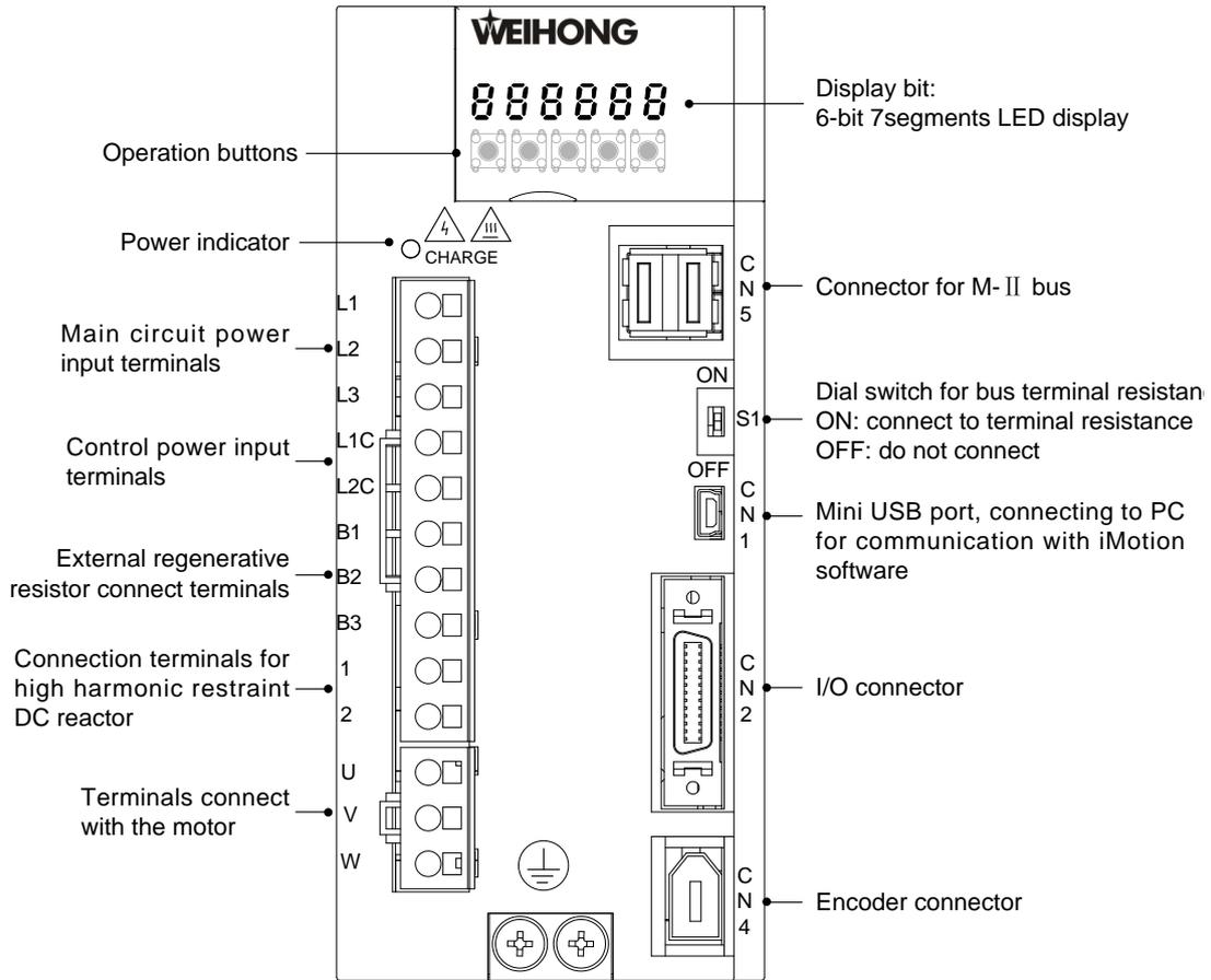
Fig. 1-2 Part description of a bus driver
