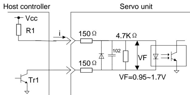
Refer to following application examples to set up the value of R1, in order to restrict current i within range of 3mA~8mA.
