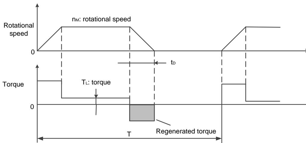
When the motor accelerate or decelerate according to the cycle shown above, the capacity of regenerative resistor can be calculated in the following steps.
