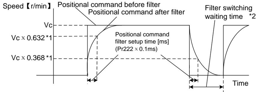
\*1: Actual filter time constant (set value  $\times 0.1\text{ms}$ ) has the maximum absolute error of 0.2ms for a time constant below 100ms and the maximum relative error of 0.1% for a time constant 20ms or more.
