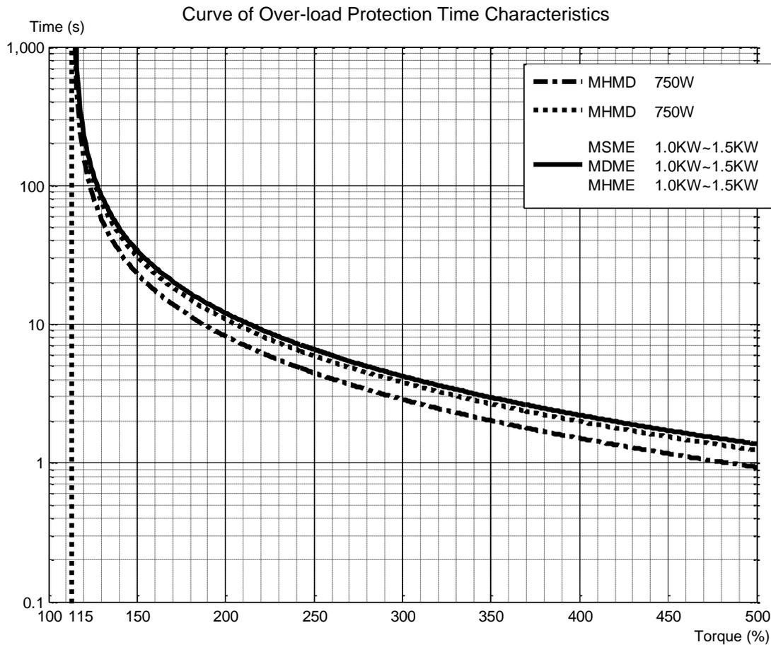
For WISE series driver 750W and 1500W, their curves of over-load protection time characteristics are the same. As shown in above figure, curve in grey color are over-load protection for driver 750W and 1500W, while curve in black color is the curve for the driver 400W.
