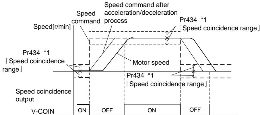
\*1: Because the speed coincidence detection is associated with 10r/min hysteresis, actual detection range is shown below.
