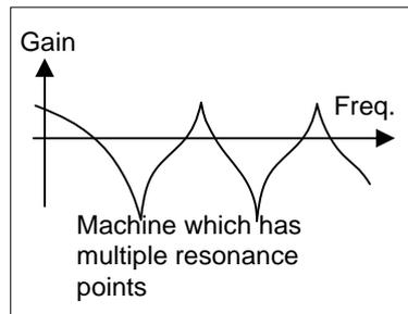
Adaptive filter and notch filter enabled
