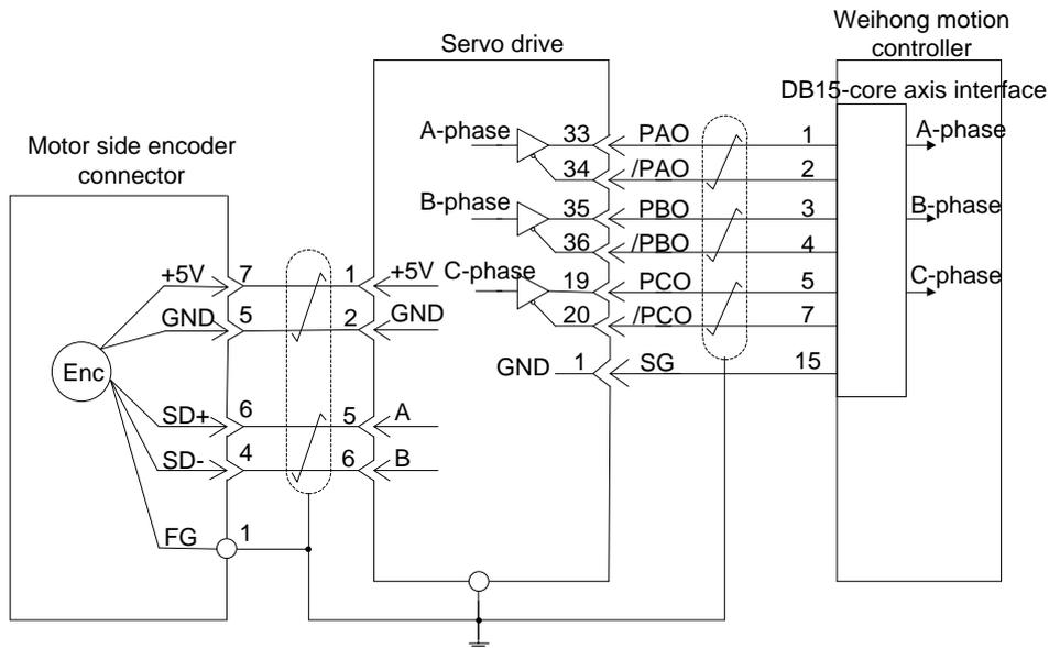
Below is the wiring diagram of MA040, MA060, MA080, MN080 and MN130 model with absolute encoder.
