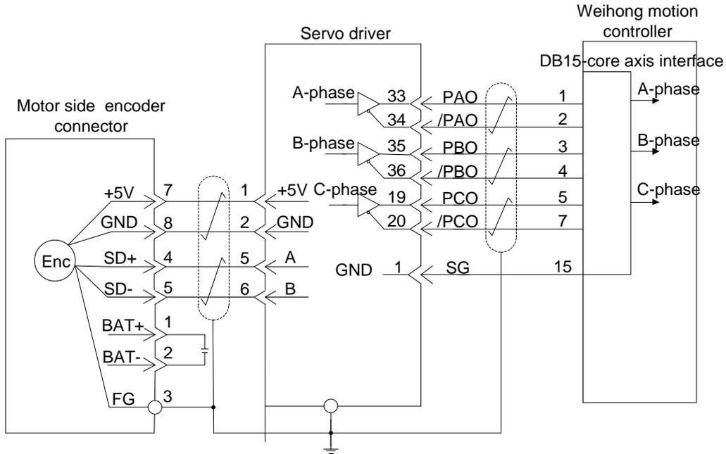
In the following figure, MDME model type of the motor (1000W and 1500W), and 17-bit absolute encoder are used.
