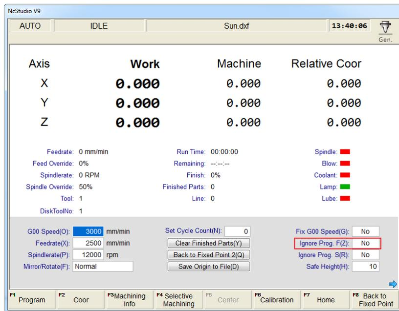
Fig. 3-53 Parameters setting zone-feedrate setting
