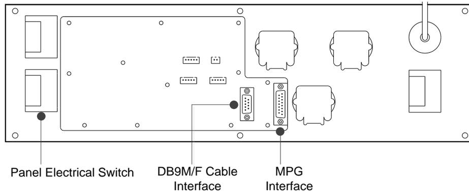
Fig. 1-11 Rear view of WH106A3 operation panel
