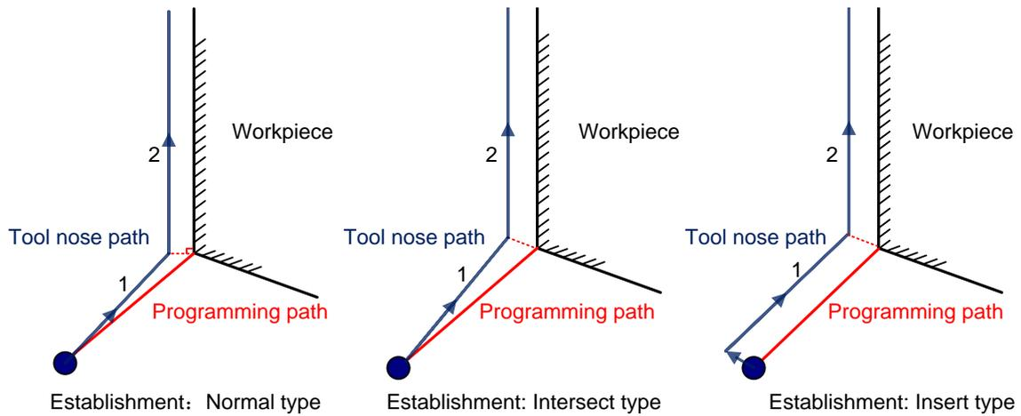
Fig. 3-64 Type to establish tool compensation
