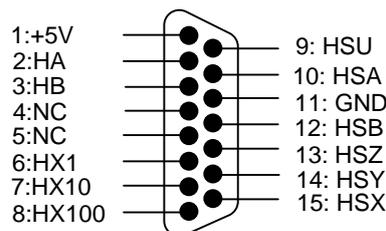
Fig. 2-14 Handwheel interface definition
